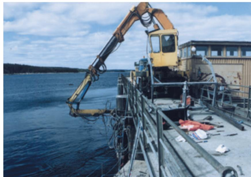
The Jetframe mounted on a carrier
