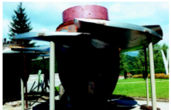
The new four blade, variable pitch, turbine.
