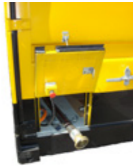
Inlet and outlet for hoses and cables, conveniently fitted through a shared hatch
