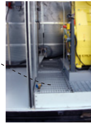
The collection tray with drain plug prevents oil and fuel spillage from polluting the worksite
