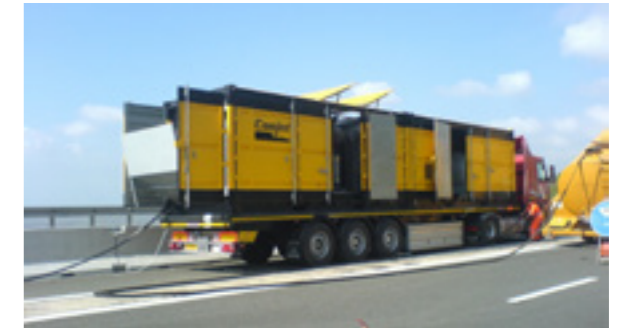
A Conjet Powerpack 540-750 kW on a trailer together with a customized service container
